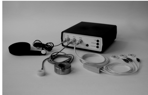
Fig. 3. BioLab STI smart sensor module with ECG electrodes, cardio microphone and piezo-electric sensor of the carotid pulse wave.
